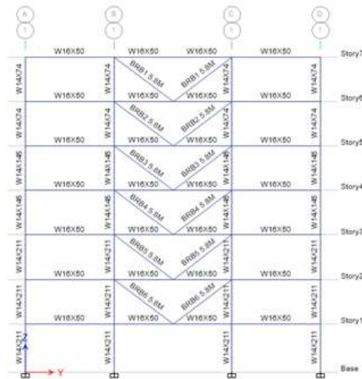
Figure 2.3. typical BF-2 elevation
